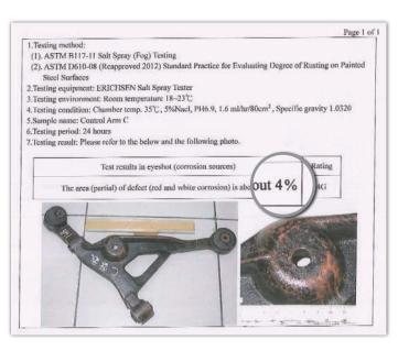
(1). ASTM B117-11 Salt Spray (Fog) Testing
